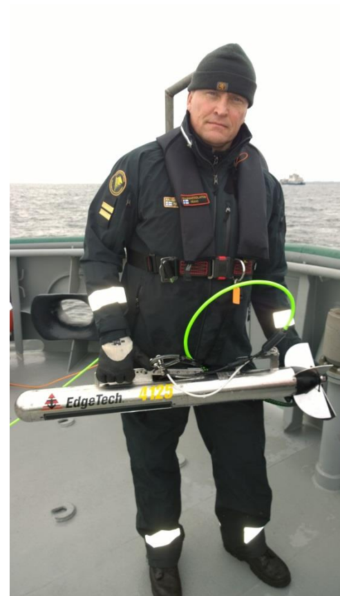
Side scan sonar tool used in Oxellösund by the Finnish Fronted Guard
